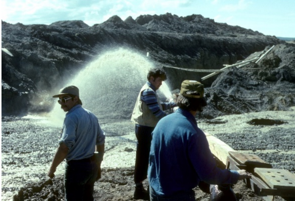
John Sims inspecting a hydraulic nozzle operating at a placer mine near Livengood, Alaska, circa 1982.
