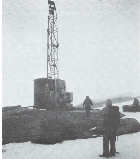
Anaconda Minerals diamond drilling platform on Red Mountain chrome deposit in 1981, from Bundtzen et al (1982).
