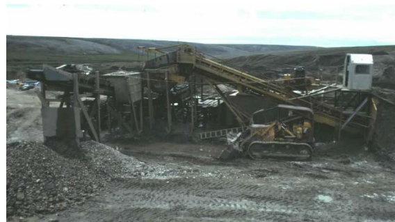
Washing plant at Len Grothe tin placer mine, circa early 1980s. Photo by Travis Hudson
