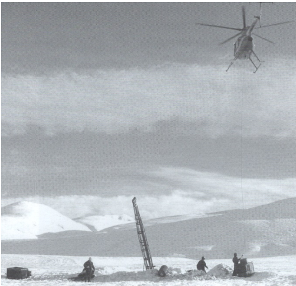
Spring core drilling at the 'MAN' nickel-copper-cobalt-PGE prospect, a part of the Fish Lake Complex; a.k.a. the original Ellis 'Nikolai' Project. Photo in Hughes and Szumigala (2006).
